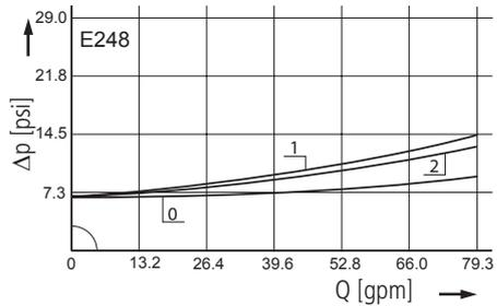
Pressure drop as a function of the **kinematic viscosity**
