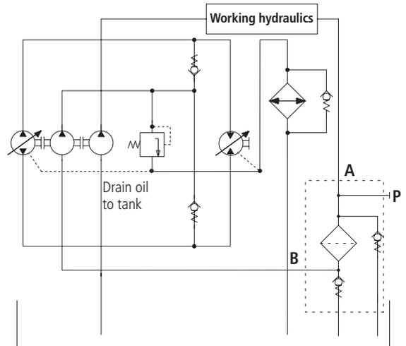
This circuit layout has the advantage that drain oil pressures are comparatively low.
