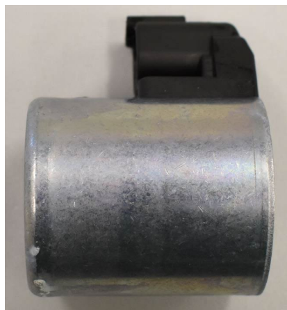
Sample after 96 h – white corrosion on the 1 % of evaluated surface
