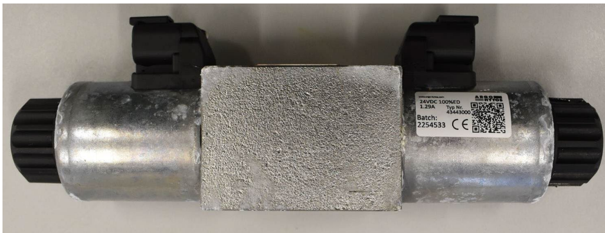
Sample after 96 h – white corrosion on the 5 % of evaluated surface
