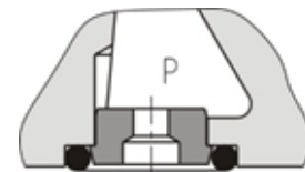
Damping nozzle (Ø 0.8 mm) at the input of the „X“ port of the pilot valve (version PF)
