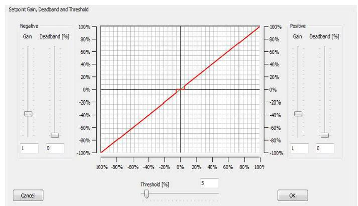
Figure 8-9: Threshold, gain and offset of the command signal
