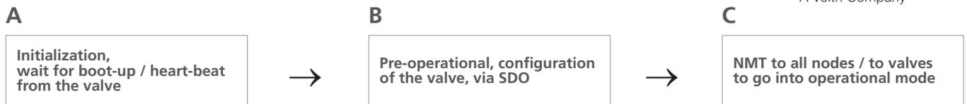
Figure 7-3: CANopen Bus initialization process
