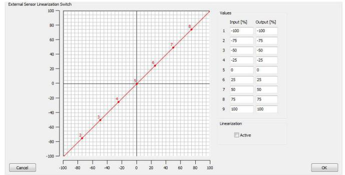
Figure 8-16: Configuration window linearization of the external sensor signal
