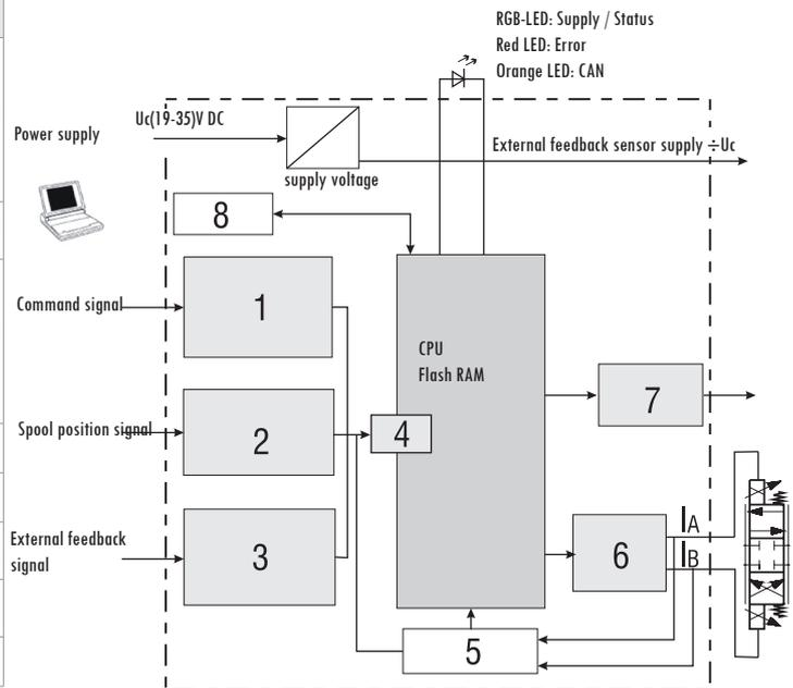
Figure 6-1: Block diagram of the digital onboard electronics
