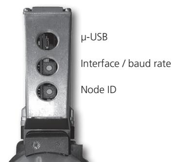
Figure 7-8: Rotary switch arrangement and designation
