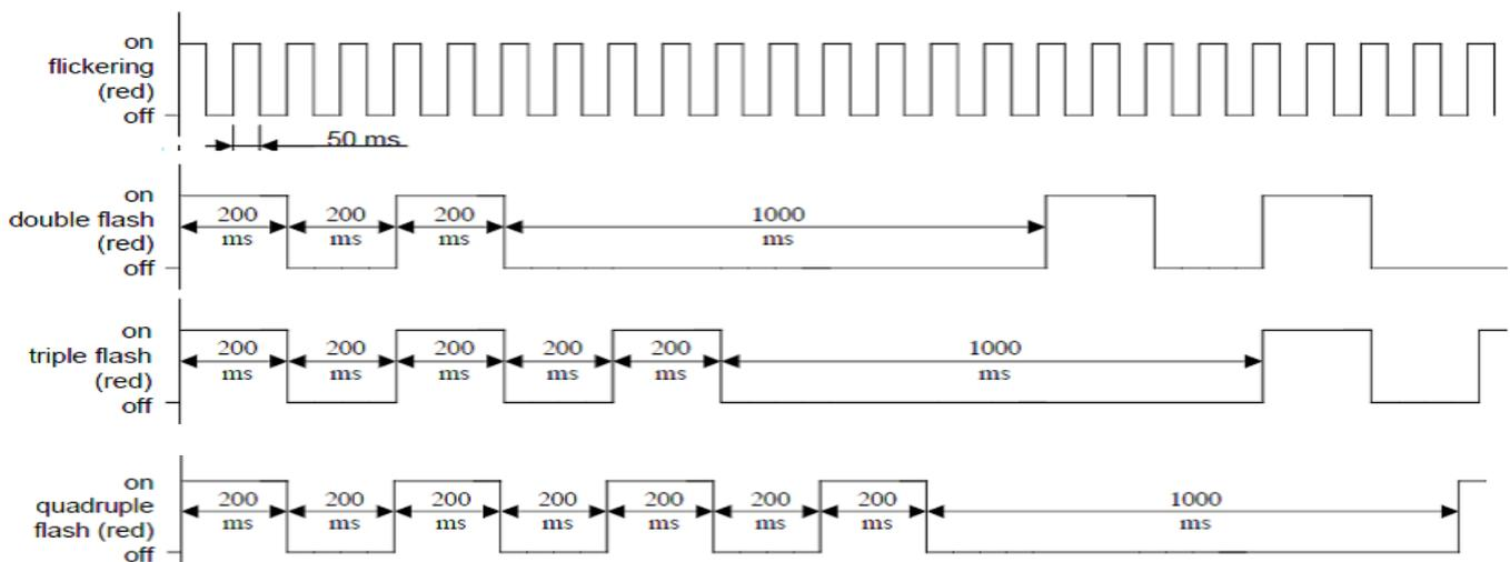
Figure 7-9: Indicator states according to CiA DS 303
