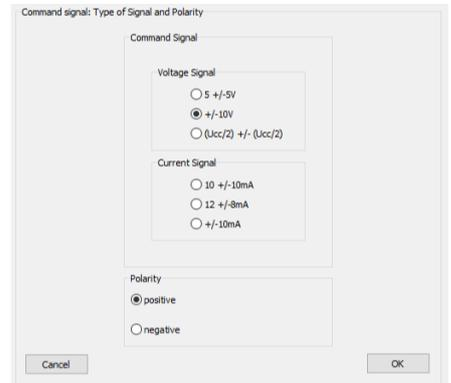
Figure 8-8: Signal type and polarity of the command signal
