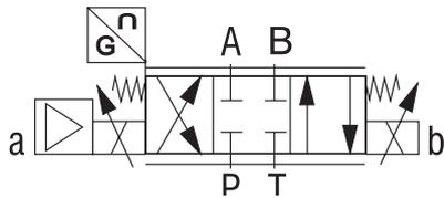
Figure 3-1: Proportional directional control valve with two coils in the configuration E02S02
