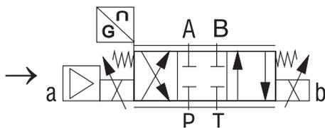
Figure 3-2: Proportional directional control valve with two coils in the configuration E04S02
