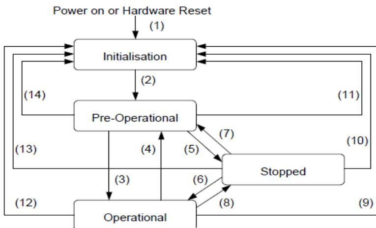
Figure 7-2: Status diagram of the CANopen protocol in the PRM9
