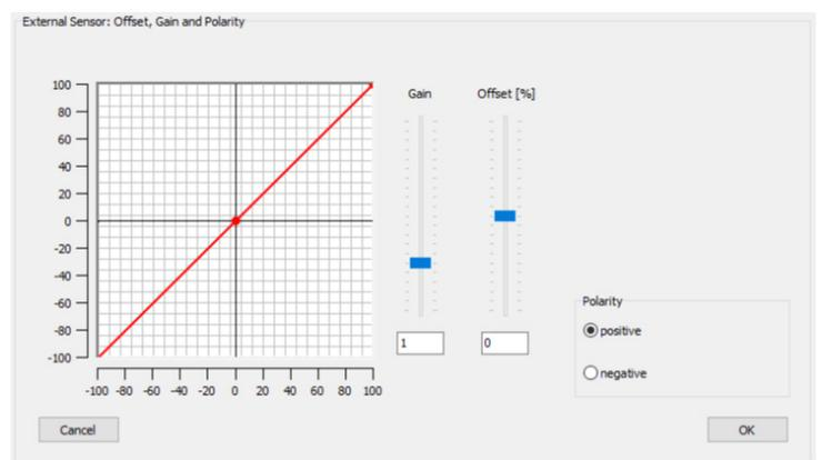
Figure 8-15: Configuration window offset and gain of the external sensor signal
