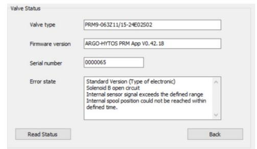
Figure 8-3 Message window of the valve status
