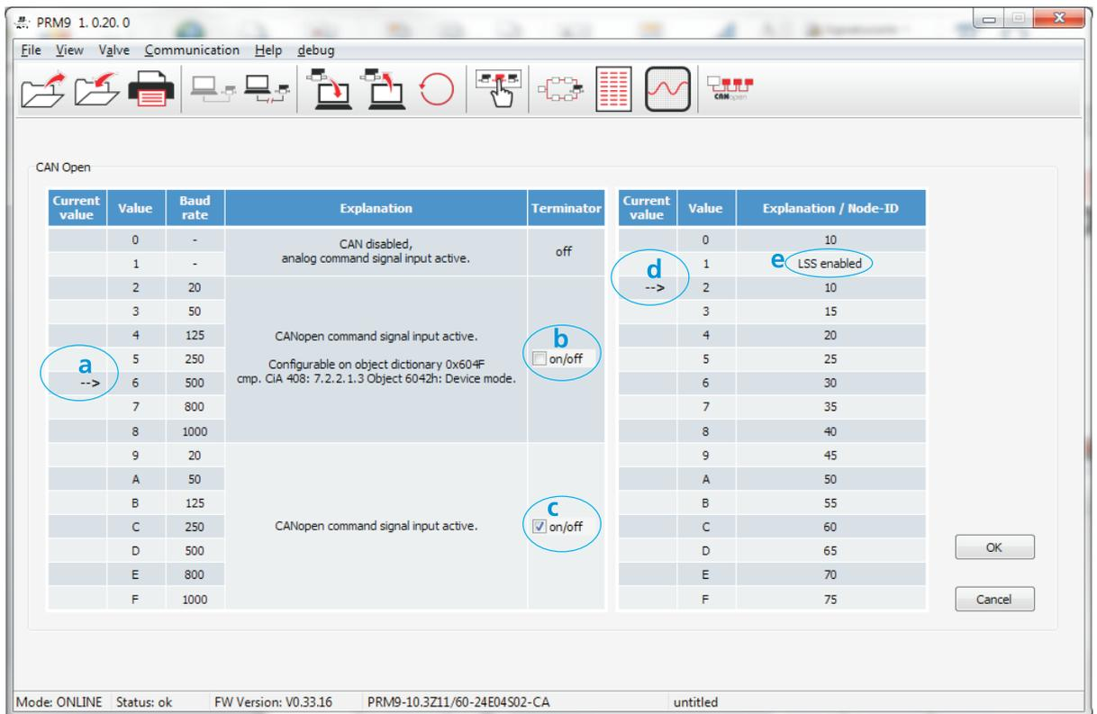
Figure 8-17: CANopen Configuration window, left table with rotary switch setting interface / baud rate, right table with setting of the rotary switch Node ID
