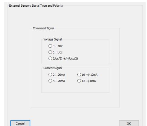
Figure 8-14: Configuration window signal type and polarity of the external sensor signal
