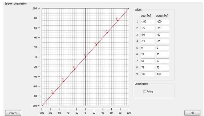
Figure 8-10: Linearization of the command signal
