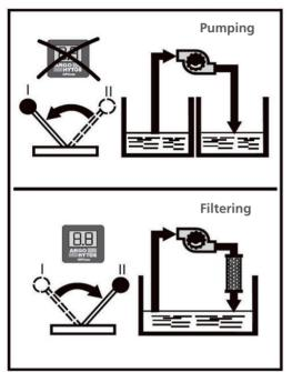
Fig. 14: Lever pumping / filtering
