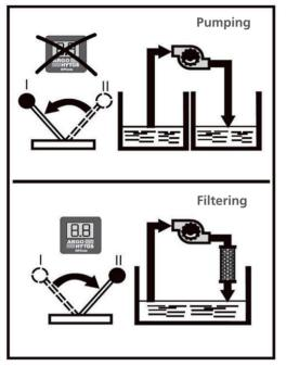
5. Set the three-way valve to the vertical position
