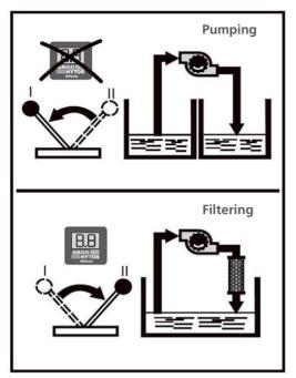
Fig. 16: Lever pumping / filtering
