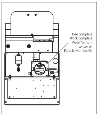
Fig. 37: Spare parts drawing 6
