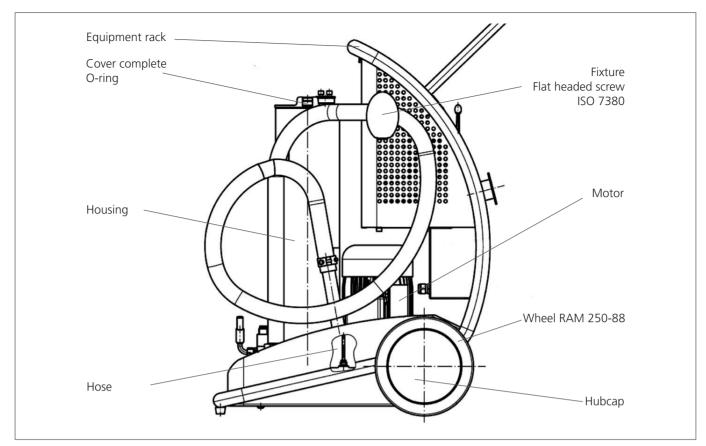
Fig. 32: Spare parts drawing 1
