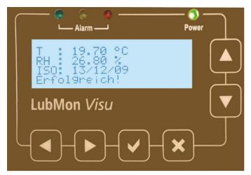
By pressing the "Hook" button, the auxiliary screen is deleted and the normal menu with the addition "SUCCESSFUL" appears.
