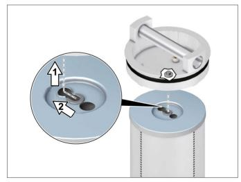
Fig. 27: Attaching the filter element
