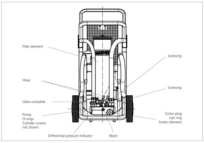
Fig. 33: Spare parts drawing 2
