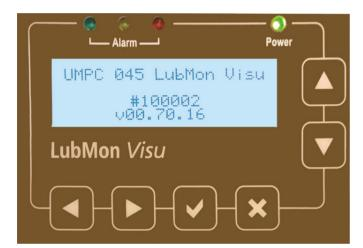
During a brief initialization phase, the display shows the version screen, which provides information about the implemented software.
