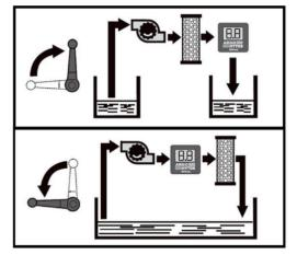
Particle Counting "Cleaning" (BEFORE filter) Fig. 20: Three-way valve
