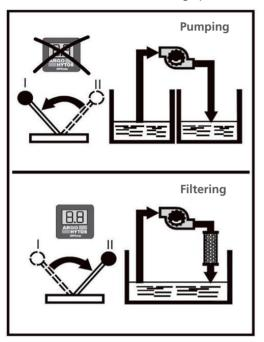
Fig. 15: Lever pumping / filtering
