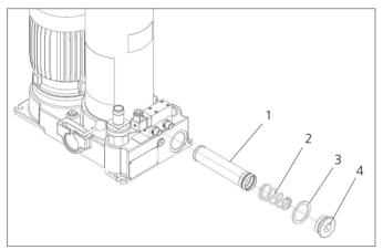
Fig. 29: Removing the suction filter
