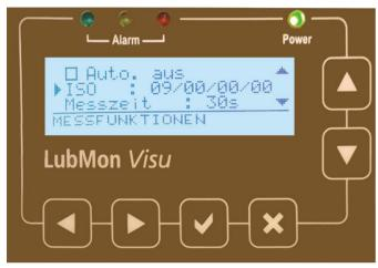
After the initialization screen (page 19, Fig. 12) has been displayed, press the "Hook" button to enter the "Automatic shutdown menu".
