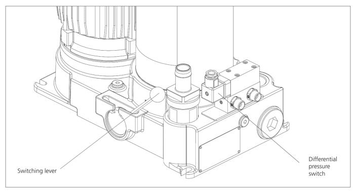
Fig.3: Component overview 3 (transport rack removed)
