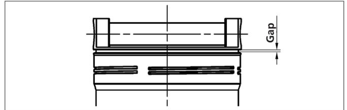
Fig. 36: Gap at the filter cover
