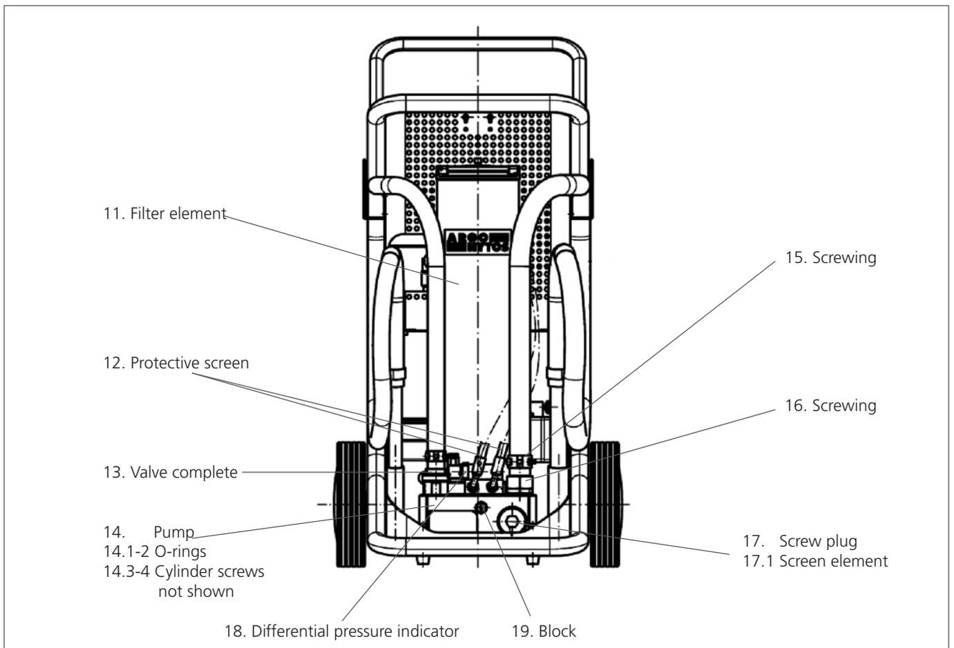
Fig. 43: Spare parts drawing 2
