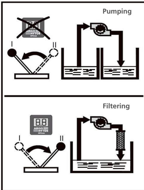
Fig. 25: Lever pumping / filtering
