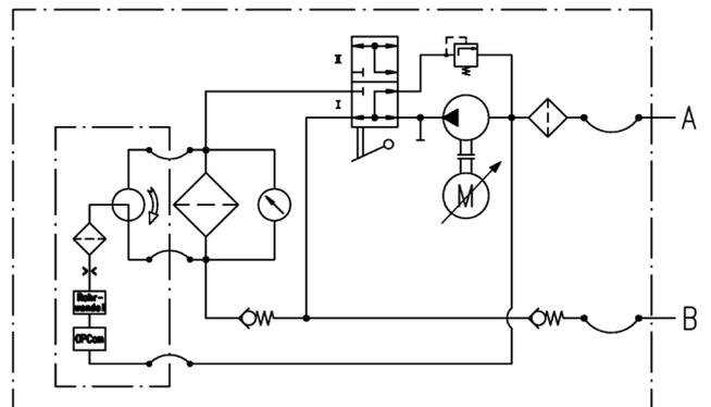
Fig. 41: Hydraulic diagram UMPC2 with variable flow
