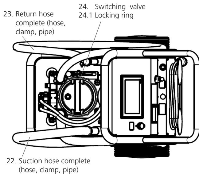
Fig.45: Spare parts drawing 4
