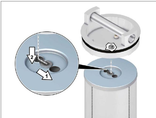
Fig. 33: Removing the filter element from the cover
