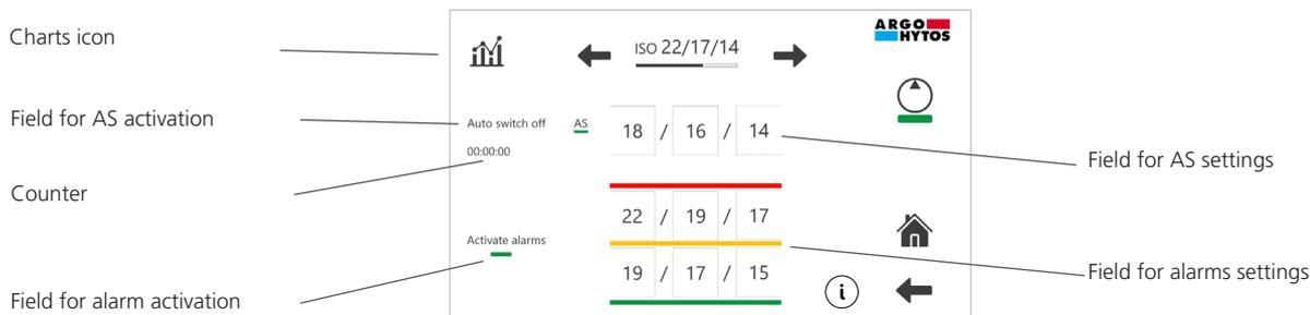
Fig. 15: Cleanliness class settings and functions
