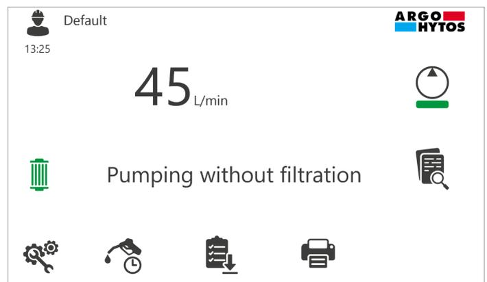
Fig. 27.1: Main screen in the "Pumping" position of the lever
