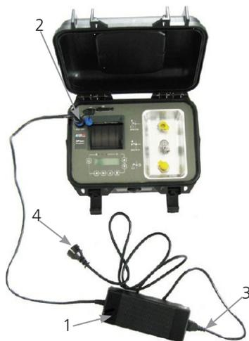
Fig. 12: Electrical connection
