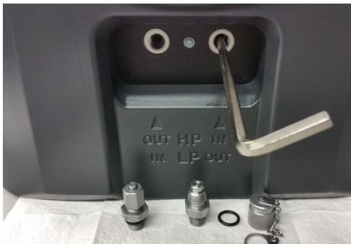
Fig. 26: Removing the protective strainer
