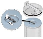
Fig. 5: Removing the filter element from the cover
