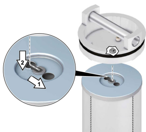
Fig. 5: Removing the filter element from the cover
