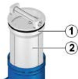
Fig. 5: Removing the filter element
