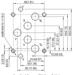
Ports P, A, B, T - max.- Ø11.2 mm (0.44 in) X,Y - max. Ø 6.3 mm (0.25 in)
