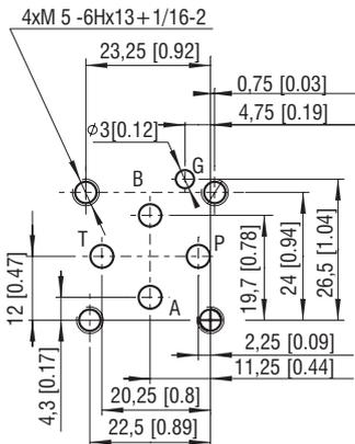
Anschlüsse P, A, B, T - max.  $\varnothing 4.5$  mm (0.18 in)
