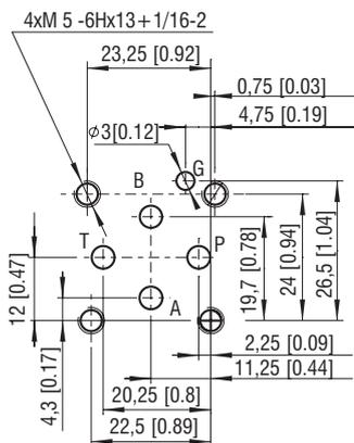
Ports P, A, B, T max  $\varnothing$ 4.5 mm (0.18 in)
