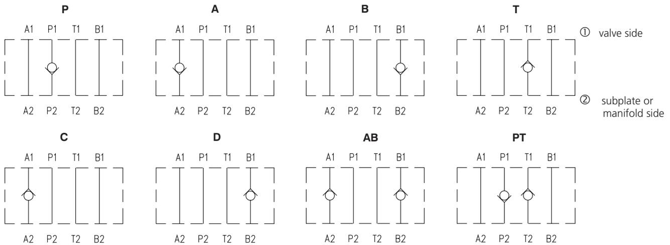
**Notes:** The orientation of the symbol on the name plate corresponds with the valve function.
