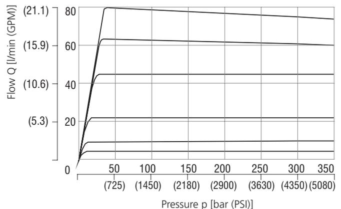
If the pressure resistance increases due to a flow rate increase, the pressure differential also has to increase in order to ensure correct regulation.
