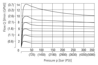
The characteristic of the pressure compensator corresponds to the flow rate of a PRM2-043Z11/12 proportional directional valve.
