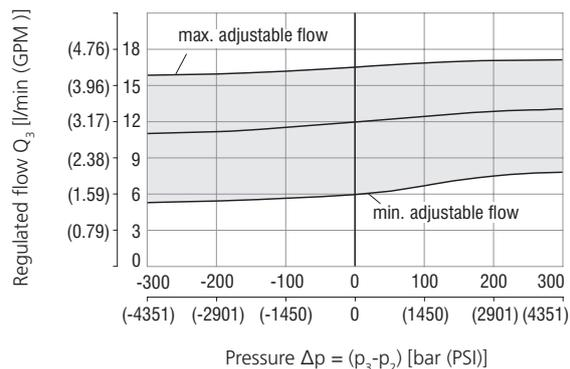
**Characteristics** measured at  $v = 32 \text{ mm}^2/\text{s}$  (156 SUS)
