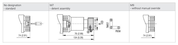
In case of solenoid malfunction or power failure, the spool of the valve can be shifted by manual override. For alternative manual overrides contact our technical support.
