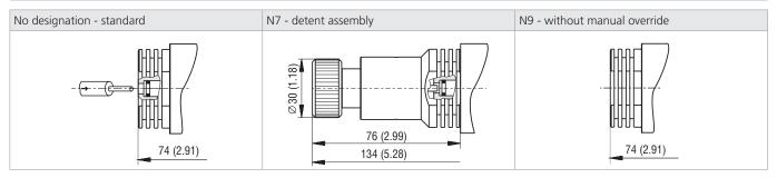
In case of solenoid malfunction or power failure, the valve spool can be shifted by manual override under the condition that the pressure in the back line does not exceed 25 bar (363 PSI).
