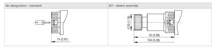
In case of solenoid malfunction or power failure, the valve spool can be shifted by manual override under the condition that the pressure in the back line does not exceed 25 bar (363 PSI).
