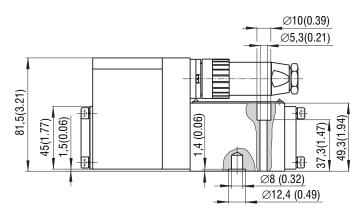
Mounting screws 8.9+1 Nm (6.6+0.7 lbf.ft) M5 x 45 DIN 912-10.9
