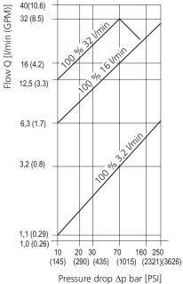
$\Delta \mathbf{p}$  = valve pressure differential (input pressure  $\mathbf{p_0}$  minus load pressure  $\mathbf{p_1}$ )
