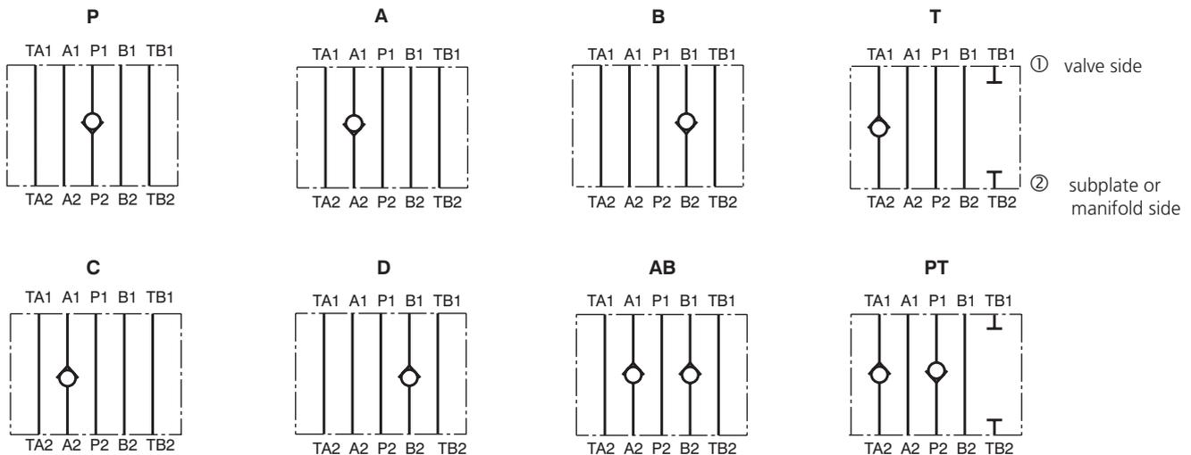
**Note:** The orientation of the symbol on the name plate corresponds with the valve function.
