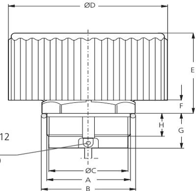
Version with thread M42 x 2 and 1<sup>5</sup>/<sub>8</sub>-12 eye R2.5 / hole Ø 2 mm / 0.08 inch
