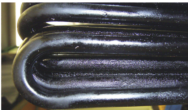
Oil aging products at tube bundles of an oil cooler
