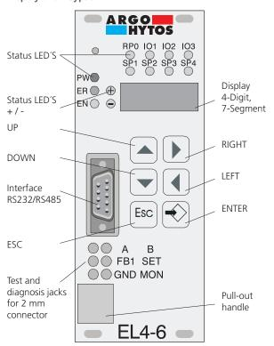
The EL4 card is multifunctional electronic control unit in Eurocard format for open and closed loop control of single or double solenoid proportional valves typically with positional feedback control. The unit controls the position of the valve spool according to the reference input signal ensuring linear regulation with minimum hysteresis. The front panel is fitted with LEDs to indicate the card functions and selectros for parametrization together with 2 mm jacks for test and diagnostics.
