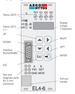
The EL4 card is multifunctional electronic control unit in Eurocard format for open and closed loop control of single or double solenoid proportional valves typically with positional feedback control. The unit controls the position of the valve spool according to the reference input signal ensuring linear regulation with minimum hysteresis. The front panel is fitted with LEDs to indicate the card functions and selectros for parametrization together with 2 mm jacks for test and diagnostics.
